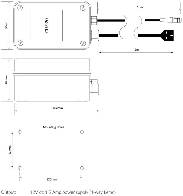
Output:12V dc 1.5 Amp power supply (4-way Lemo)Input:100-240Vac 50/60Hz (options include 16A, UK, EU, AUS, US)IP rating:IP67Fuse output:F1.5A quick blow, Ø5 x 20mmCable length:Mains cable 2m, 12Vdc 10m
