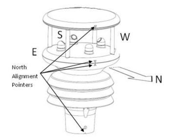
To mount the weather station or windspeed sensor to a pole, an optional pole mount bracket can be purchased (BK:902), which is suitable for poles with diameters between 30 and 58 mm (1.2" – 2.3"). The weather station should be secured to the bracket with screws (torque screws to 1.5 Nm maximum). Mount the bracket to the pole using the clamp nuts (torque set to 3 Nm).
